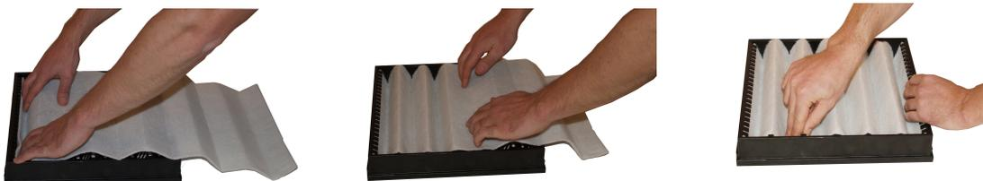
Turn the “soft” surface outwards and the “hard” surface towards the HEPA filter.
